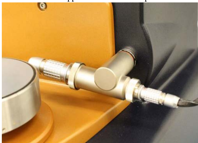
Figure 5 Connection of the UHP adapter to the Smart Swap socket (DHR Series shown).
